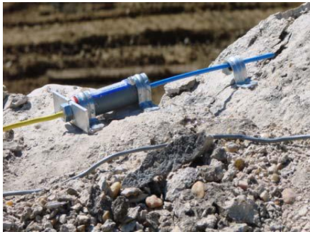
Fig 9: A d-GMM monitoring a crack in a dam buttress.
