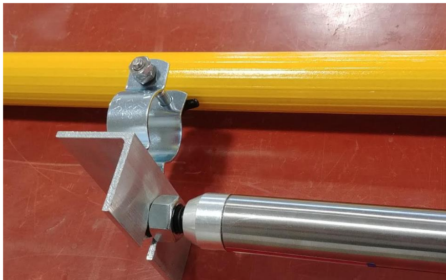
Bracket mounted on sensor to clamp to the large diameter side of the telescoping pole.
