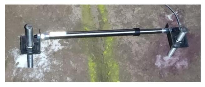
dCONV with a 200mm stroke and a 10 micron resolution
