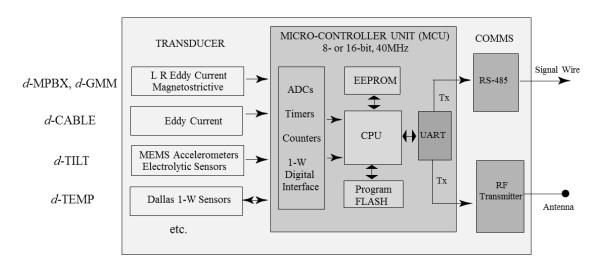
**d-Tech** Instrument architecture involves interfacing a myriad transducer technologies (some SMART digital, some analog) with an embedded microcontroller running at 40MHz, and an output transceiver, usually RS485 or Zigbee wireless.
