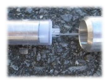
Cut off that rod with a sharp cutting tool.
