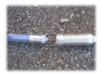
You can now see the thin metal rod used for the readings in that distal extensometer segment.
