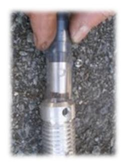
Secure the plug back in place by tightening the set screw
