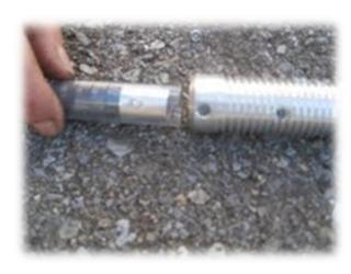
Go to the previous (second distal) anchor point and start unscrewing the bolt located distally (near the toe and near the segment to be removed) on that anchor).
