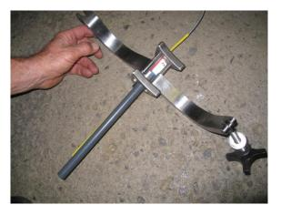
Step 3: Clamp the displacement sensor to the cylinder.
