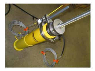
It is of paramount importance that the load cell be inserted between the two flat platens. Failure to compress the load cell between two flat surfaces may result in inaccurate readings. Eccentric loading may also result in inaccurate load cell reading. Always compare load cell reading with the pressure in the line multiplied by the area of the cylinder.
