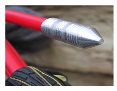
The distal anchor point is tapered to facilitate insertion into the borehole.
