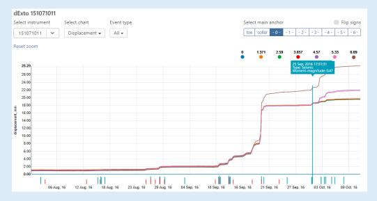
This software features a very powerful zooming capability that allows engineers to analyze the effect of individual blasts or seismic events. By establishing relationships between the magnitude and distance (concept of scaled distance) of events and the corresponding "micro-damage" to the walls of excavations, powerful predictive models can be developed.
