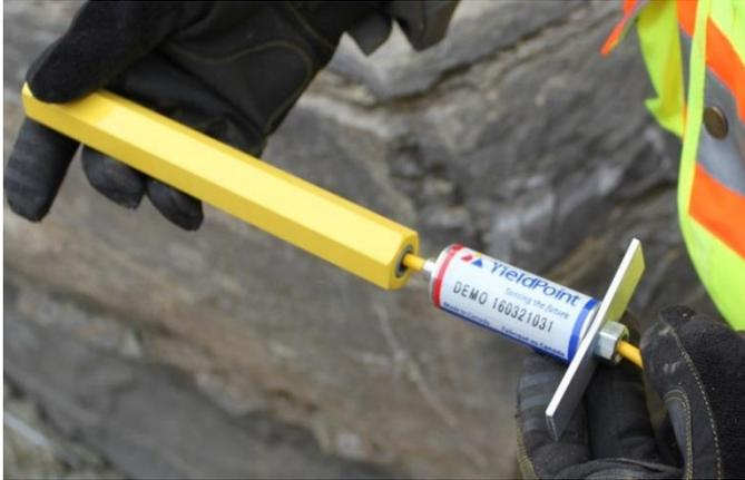
YieldPoint's **d-GMM(SPECTRE)** displacement sensor integrates magnetostrictive technology to produce a high precision digital instrument comprising a non-contact displacement sensor and digital temperature sensor. An on-board microcontroller applies temperature compensation and outputs a digital signal. Both the resolution (<0.01mm) and accuracy (0.25% linearity typical) are significantly better than for similarly priced technology.
