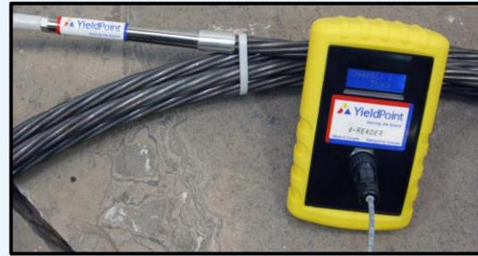
Measurements are output from the instrument directly in mm according to the d-tech format. The RS485 output signal can be transmitted over 500m without amplification. These values represent the stretch of the steel cable. As a quick conversion to load, 8mm of differential stretch between adjacent nodes results in 240kN of load for a 1m node spacing.
