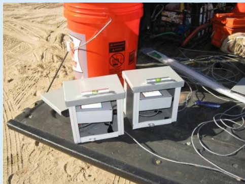
2 x d 2 TILT-EL tilt sensors about to be installed on a bridge in Florida, US, by engineers from Sauls Seismic Inc.
