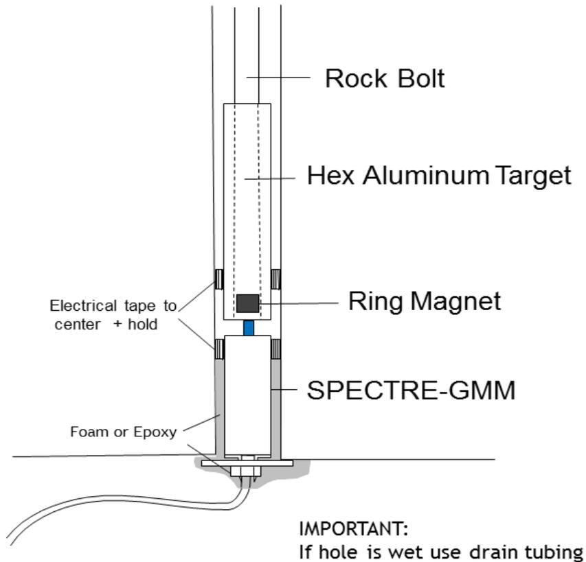
Install the d-GMM so that it has a initial reading of around 15mm. The aluminum faceplate can be omitted.
