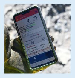
The BluLink enables instruments to be managed by an Android device using the BluPoint App. The ViewPoint activity allows the Android device to act like a manual readout unit. The LogPoint activity configures and operates the data-logging functionality of the BluLink. The BluLink 'beacons' its readings every 5 seconds to any Gateway or Logger device with 100m range.
