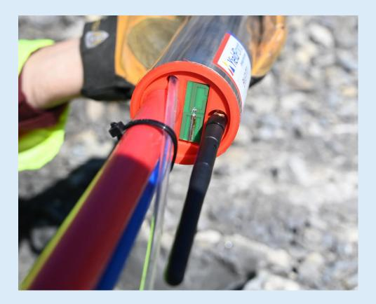
For monitoring of backs and hanging walls in blasthole stopes various options exist to enable BluEXTO to survive during stope blasting. The data logging functionality allows stored data to be downloaded by a gateway device after some degree of access becomes available.
