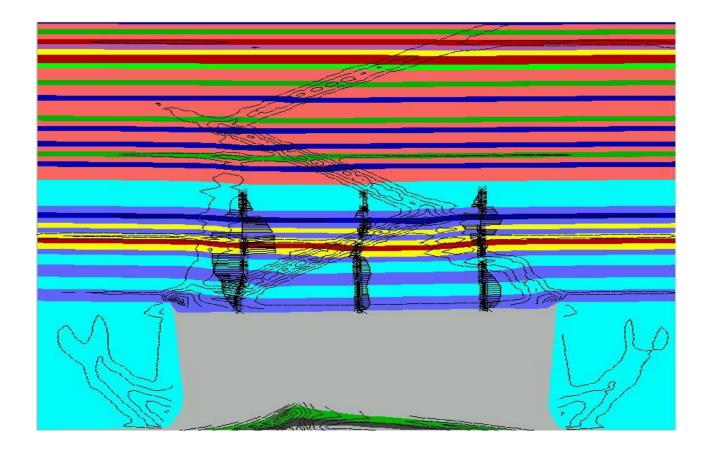
Independently conducted FLAC modeling [17]. The model uses strain softening behavior of failed rock to simulate "shear bands" similar to those hypothesized by the instrumentation results.
