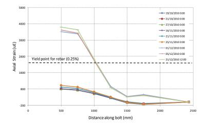
In reality it is found that loads quickly transfer onto the rebar's bolt plate depending upon the proximity of the deformation to the collar.
