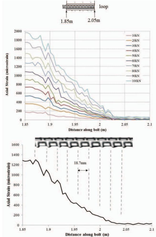
**Figure 5. Detailed axial strain profile for the bonded section of the bolt (1.85m to 2.05m along the fiber). Upper: Change in strain profiles with the applied axial load. Lower: Detailed variation of axial strain (at 70kN) related to rib geometry.**
