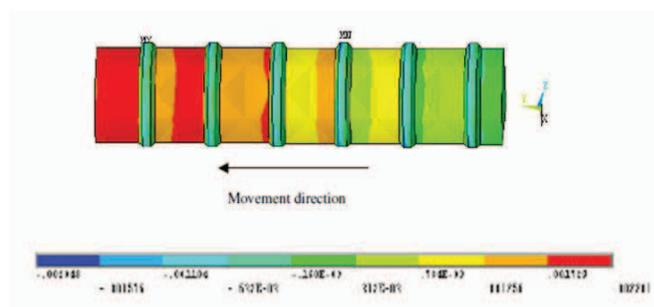
**Figure 6. Simulation of the strain profile caused by ribbing using ANSYS FE program by Jalalifar(2006).**
