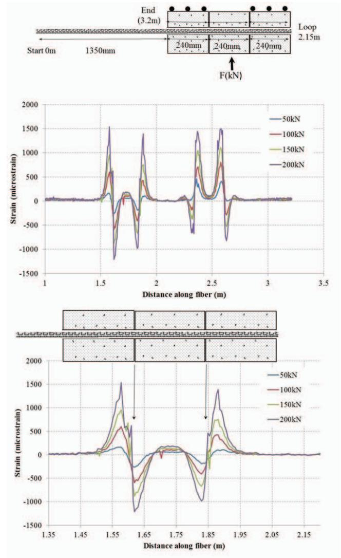
**Figure 8.** Results from the double shear test. The applied load in KN corresponds to the load-displacement profile in Figure 9. Upper: configuration. Middle: Strain profile along whole fiber. Lower: detailed Strain profile along a detailed section of fiber.
