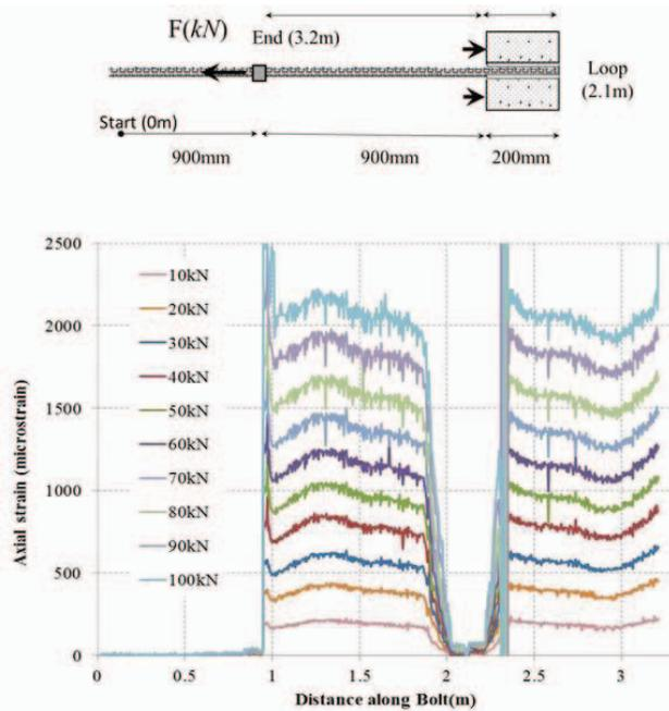
**Figure 4. Axial pull test results. Upper: Configuration. Lower: strain profile along whole fiber length.**
