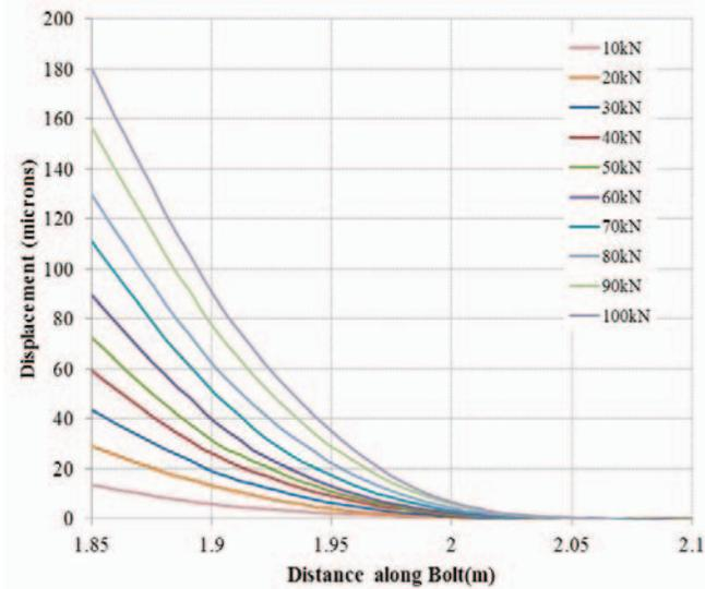
**Figure 7.** Experimental displacement profile based on integration of the strain profile in Figure 5(upper). Note: These are experimental results.
