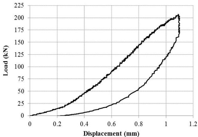
**Figure 9.** The load-deformation response of the Double Shear specimen. The load(kN) was applied to lower surface of the central block. Displacement(mm) is the relative movement between the central block and the outer blocks.
