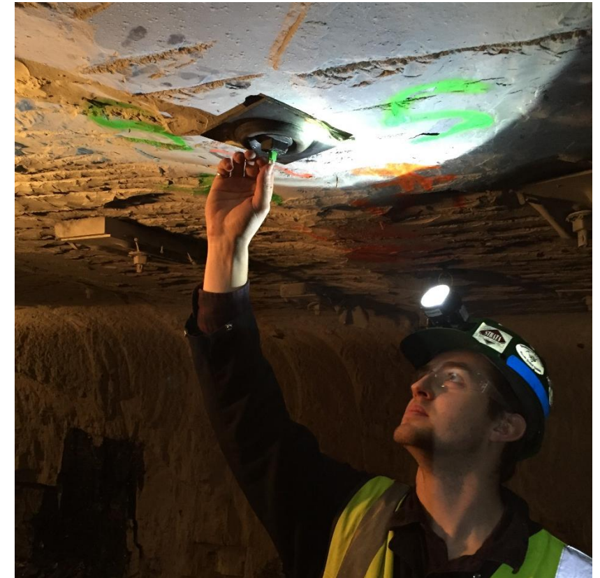
DOS instrumented bolt installed in the roof of a coal mine
