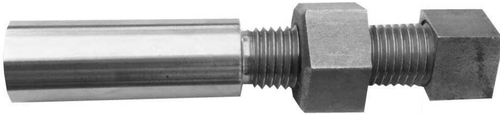
Figure 2: The U-cell. Typical diameter is 31mm in for 16mm or 19mm rock bolts, and is 35mm diameter for 22mm rock bolts.
