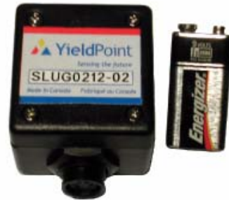
Figure 6. The SLUG data-logger
