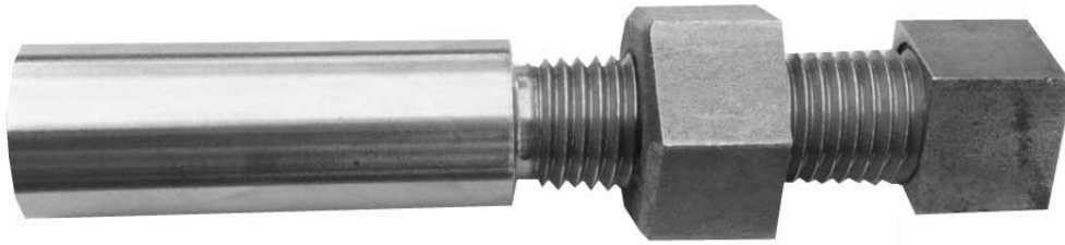
Figure 2: The U-cell. Typical diameter is 31mm in for 16mm or 19mm rock bolts, and is 35mm diameter for 22mm rock bolts.
