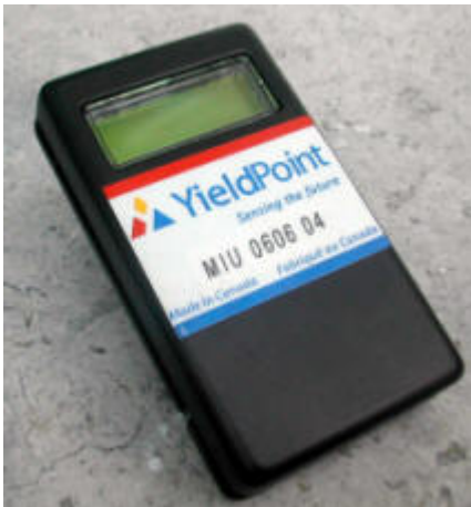
The manual readout unit. The LCD is backlit for underground
