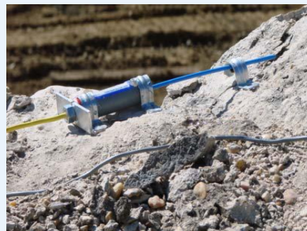
A SPECTRE GMM monitoring a crack in a dam buttress.
