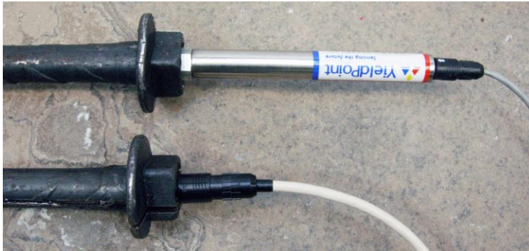
Fig 1: The two configurations for d -REBAR
