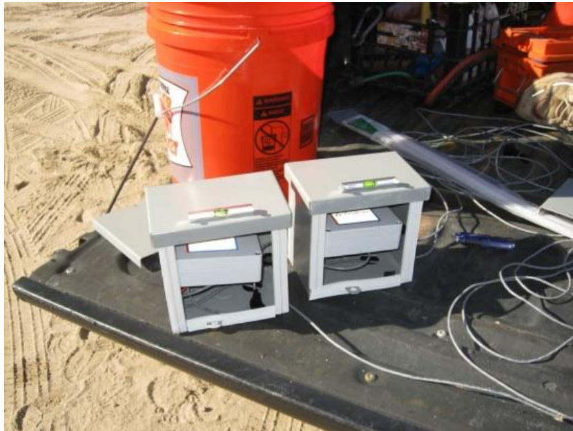
d -TILT (EL) sensor being prepared for installation on a bridge in Florida(US) by Sauls Seismic Inc.
