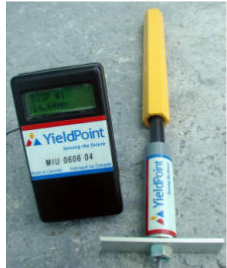
The DETECT GMM and manual readout unit. The output is directly in mm with a resolution of 10 microns
